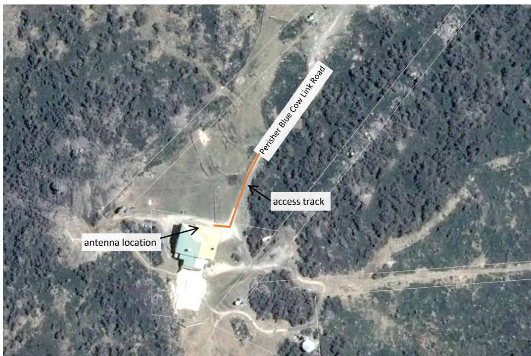
Figure 8: Proposed facility access track
